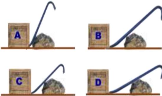
In which one of A, B, C, and D would the crate be most difficult to move with the crowbar?
