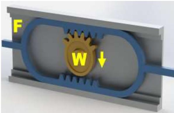
W is a wheel with teeth on part of its edge. F is a frame which can move sideways in its bearings. If W continuously turns clockwise, as shown by the arrow, F will move:
