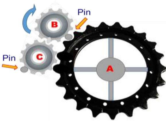
Wheel B turns and drives wheel C. B and C both have pins which fit into the slots to turn wheel A. If B continuously turns clockwise, as shown by the arrow, A will:
