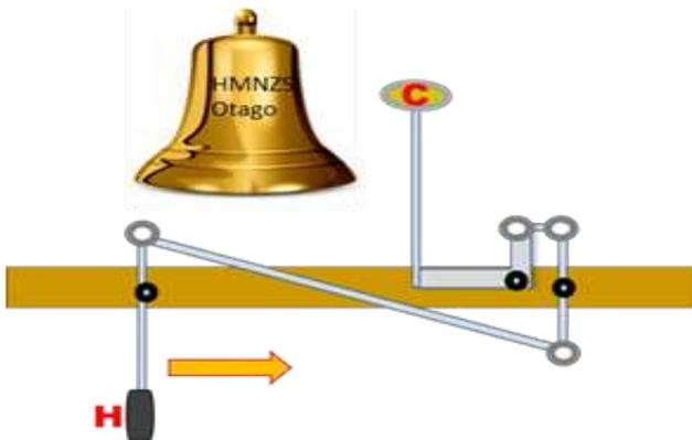
When handle H is pulled to the right, as shown by the arrow, clapper C will move:
