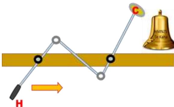
If handle H is pulled to the right, as shown by the arrow, bell clapper C will:
