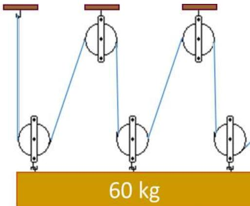
How much force is required to lift the 60 kg wooden beam?
