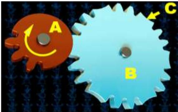
If wheel A makes 10 complete turns, how many times will point C on wheel B come into contact with A?
