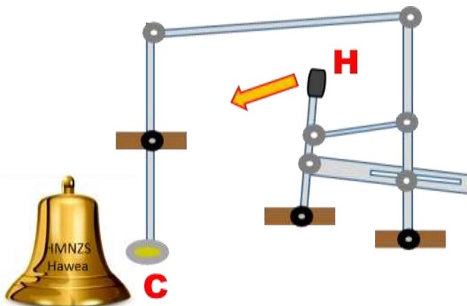
If handle H is pulled to the left, as shown by the arrow, clapper C will move:
