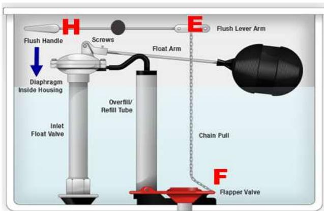
If handle H is pulled down, as shown by the arrow, how will ends E and F move?
