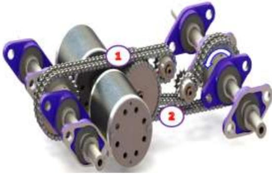
1 and 2 are attached to the chain which runs around this vertical system of wheels. If the drive shaft moves the chain down, as shown by the arrow, how will 1 and 2 move?
