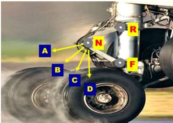
As non-fixed pivot R moves down the RNZAF 757 landing gear towards non-fixed pivot F, what path will non-fixed pivot N follow?
