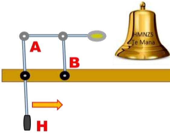
If handle H is pulled to the right, as shown by the arrow, how will the bell clapper move?
