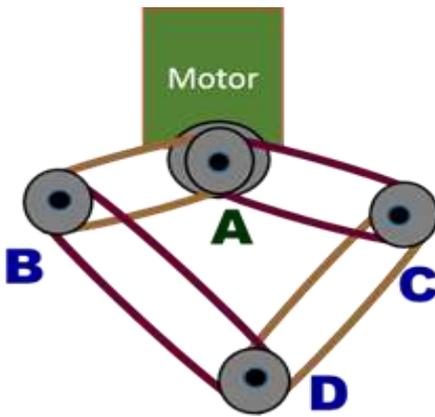
This mechanism, in which the motor A uses belts to drive wheels B, C and D is:
