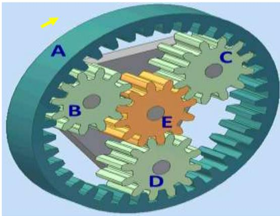
Gear A turns clockwise, as shown by the arrow, and drives all the other gears. How many gears turn clockwise in total?
