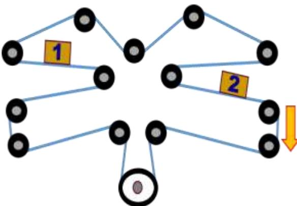
1 and 2 are crates attached to the wire which runs around this vertical system of wheels. If the wire is pulled down, as shown by the arrow, how will 1 and 2 move?
