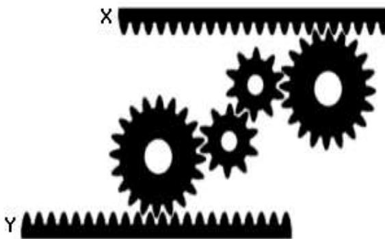
If bar Y moves right at a constant speed. How does bar X move?
