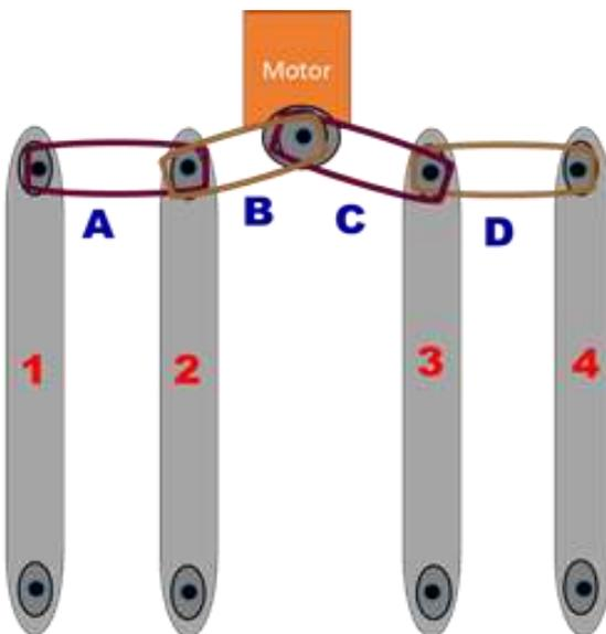
In an airport baggage handling area, the motor in the middle uses belts A, B, C and D to drive the 1st, 2nd, 3rd and 4<sup>th</sup> baggage conveyors. If the 3rd and 4th conveyors are turning but the 1st and 2nd conveyors are not turning, which one of the belts is most likely to have broken?
