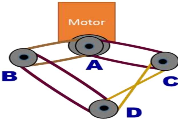
This mechanism, in which the motor A uses belts to drive wheels B, C and D is:
